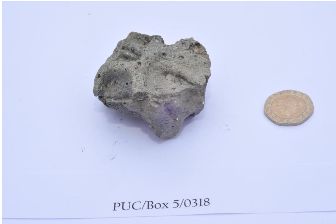
Plate 8: Melting, vesiculation and charcoal casts
