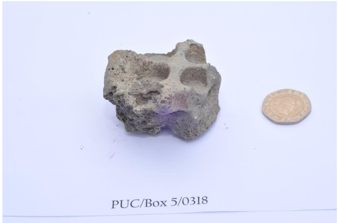
Plate 9: Differential heating of edge and centre of a tray
